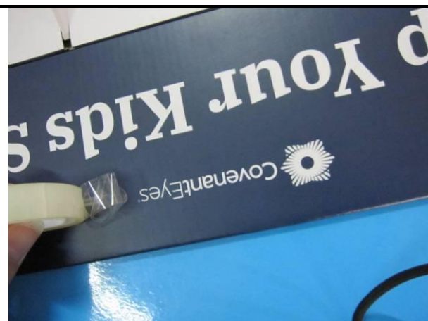
106. 3M tape test for printing—pass
