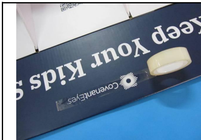
105. 3M tape test for printing—pass
